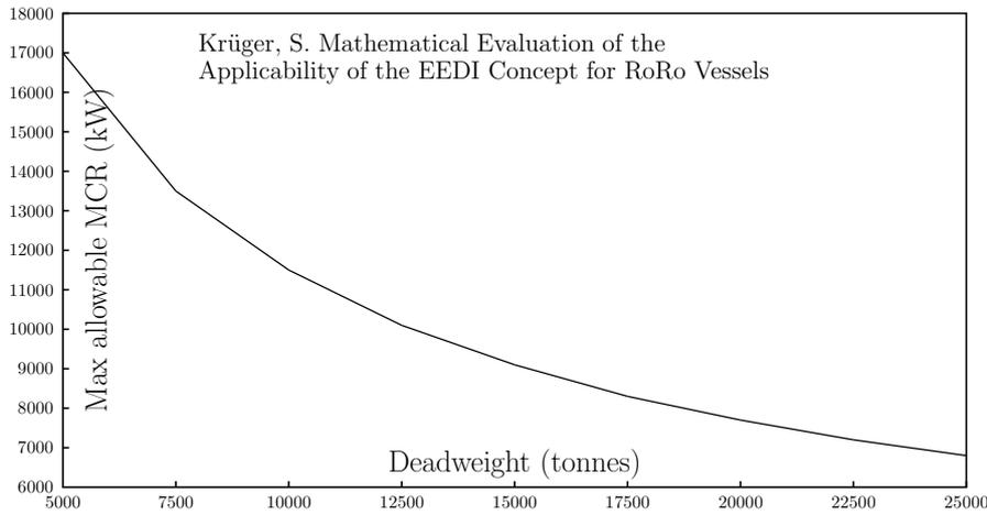
Figure 1: Allowable MCR for RoRo Ships under EEDI
